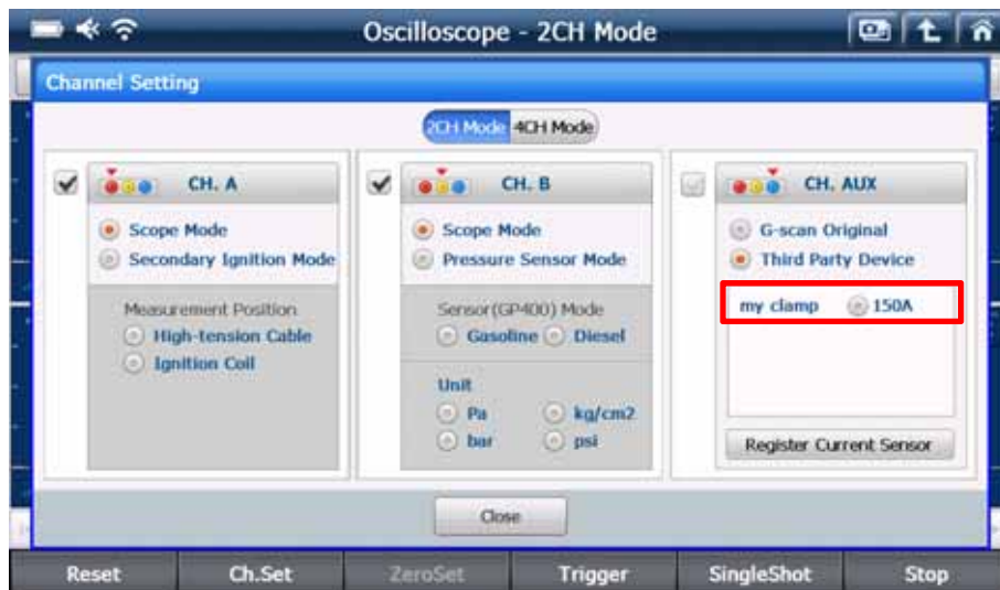
[ Channel Setting – Third party Current Sensor Registration Completed ]
